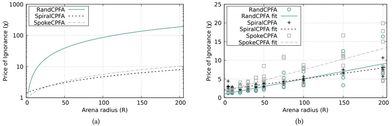
Fig. 3: (a) Comparison of CPFAs from formal analysis. Note that the y-axis is on a log scale. (b) Price of Ignorance for simulated robots ( $N = 10$ ). Collisions cause the SPIRALCPFA to underperform for smaller arena sizes.
