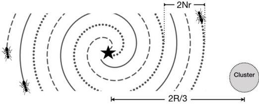
Fig. 1: Foraging path for  $N = 3$  bots using SPIRALCPFA, with a cluster placed at the expected distance of  $2R/3$  from the collection zone.
