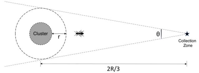
Fig. 2: Relationship between the angular region in which the cluster is detected in a single ballistic walk and the area of the cluster/ detection radius of the robot.
