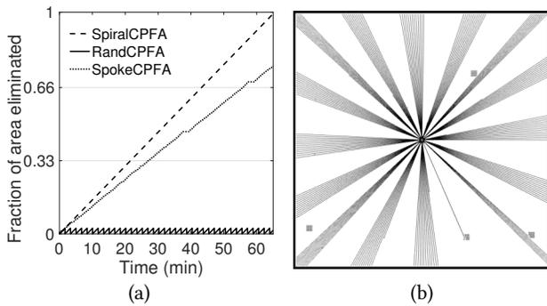
Fig. 5: (a) Fraction of area explored by the robot over time. SPIRALCPFA never re-searches the same area, which reduces the price of ignorance. (b) Visualisation of SPOKECPFA in ARGoS. Black lines are drawn where robots have searched. A gradient is visible showing that areas near the nest have been re-searched multiple times.
